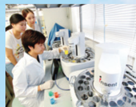
Research and Development Center for Taste and Odor Sensing: R&D TAOS - Taste sensors to detect and identify flavor (a world-first invention)
